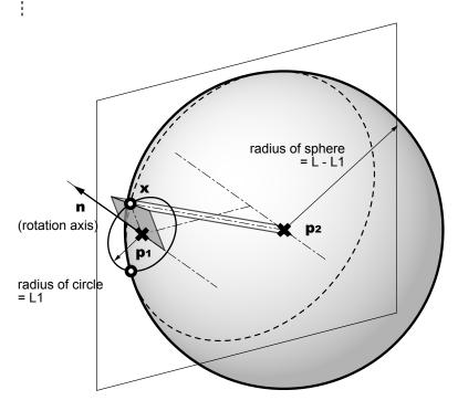
When end points of folded panel **p1** and **p2** are given, and panel length L and distance from the end point **p1** to folding point **X** is specified, folding point **X** in 3D is provided by intersection of a circle whose center is **p1**, radius is L1 and normal is rotation axis n and a sphere whose center is **p2** and radius is L-L1.
